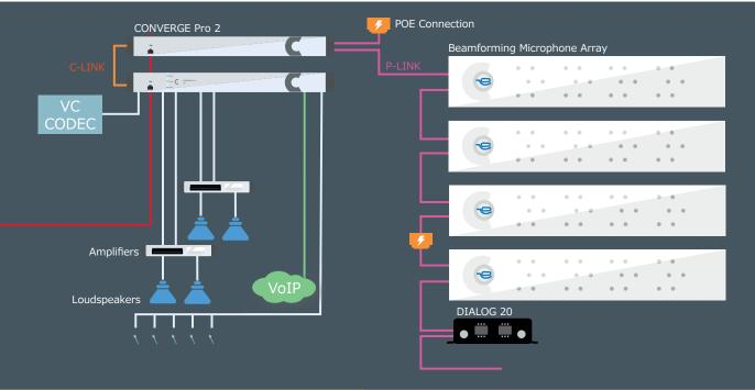
C-LINK gives you a scalable system. Units can be stacked together in any combination
