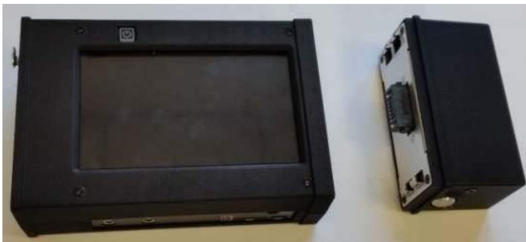
Picture 8: Codec + battery bloc split off
